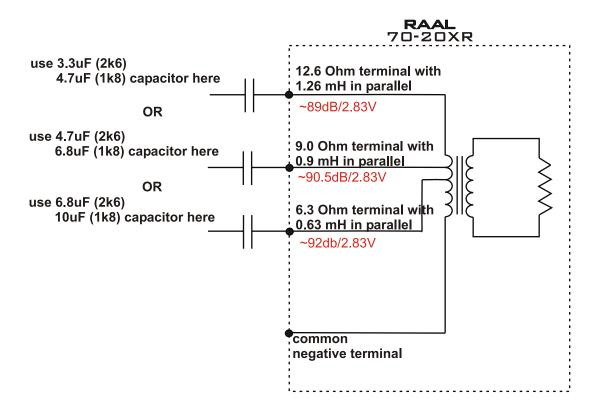
This tweeter has a built-in inductance with a set value. It's impedance matching transformer is a part of the filter.
